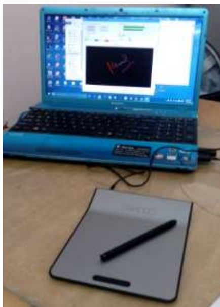
Fig1: System with digital tablet for signature acquisition
